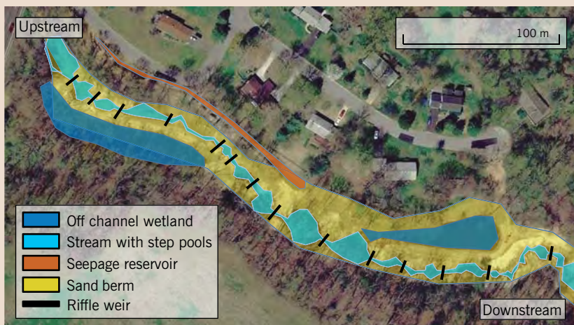
Figure 11.8: Wilelinor stream-seepage wetland site design, incorporating a combination of wetlands, step pool structures, sand berms, and weirs to slow storm velocities, promote floodplain wetland connectivity, increase hydraulic retention, reduce erosion, and improve water quality (38.967978 N, 76.544738 W, Annapolis, Maryland, USA)
